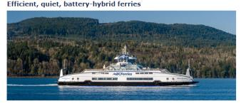
The Island Class are battery-equipped ships designed for full electric operation. The ships are fitted with hybrid technology that bridges the gap until shore charging infrastructure becomes available. From the exterior details to the engines, the design of the new vessels reduces underwater radiated noise, lowers emissions and improves the customer experience on board.
