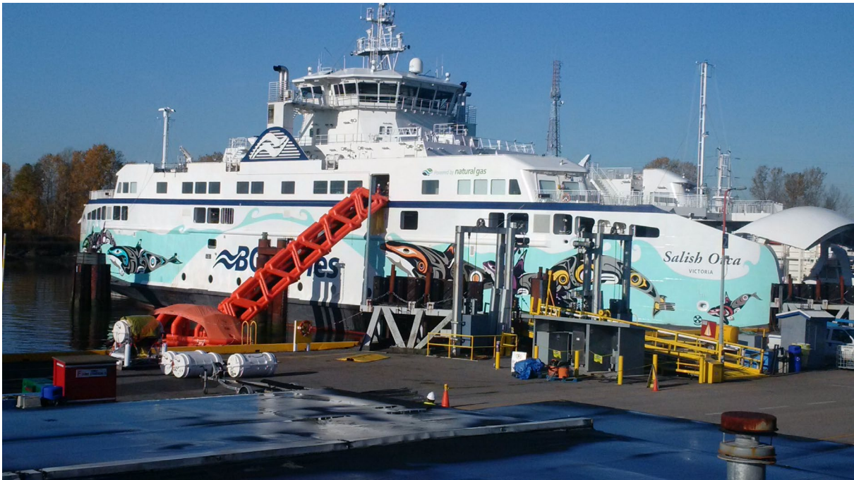
The LSA slide deployed on the Salish Orca during her refit at Fleet Maintenance Unit.
