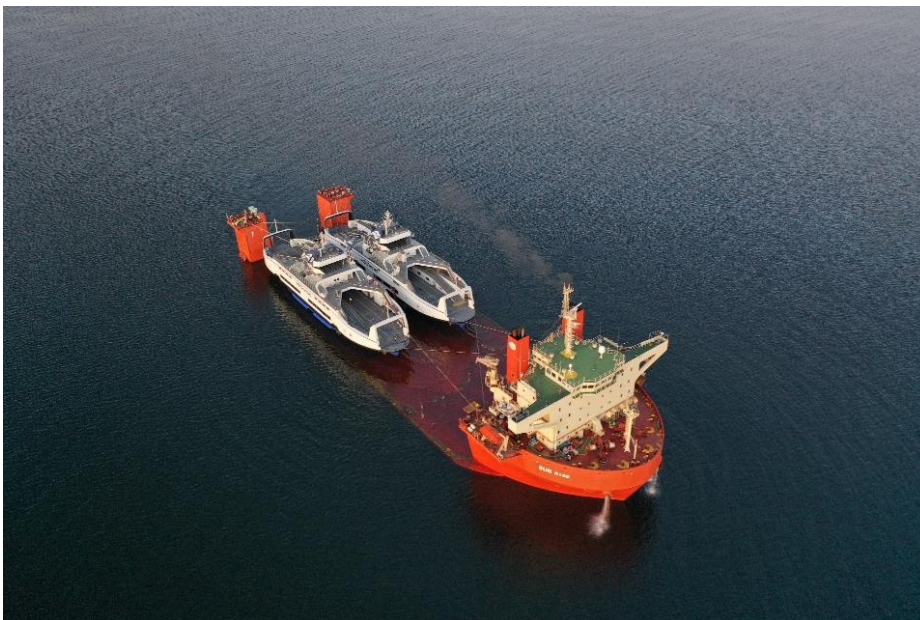
Constanta, Romania – Both ships in place on the semi-submersible transport ship.
