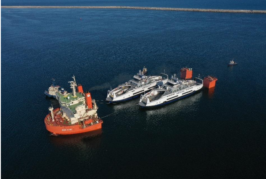
Constanta, Romania - A tugboat assists putting the Island Class ships in place while the semi-submersible transport vessel is partially submerged.
